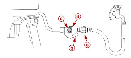
Flush the internal water passages of the outboard with fresh water after each use in salt, polluted, or muddy water. This will help prevent a buildup of deposits from clogging the internal water passages.
