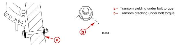
Use a dial torque wrench to determine transom strength. If the bolt or nut continues to turn without the torque reading on the dial increasing, it is an indication that the transom is yielding. The load area can be increased by using a larger washer or a transom reinforcement plate.
