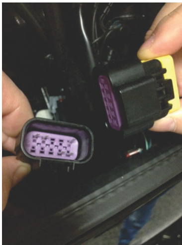
10-pin connector on the engine
