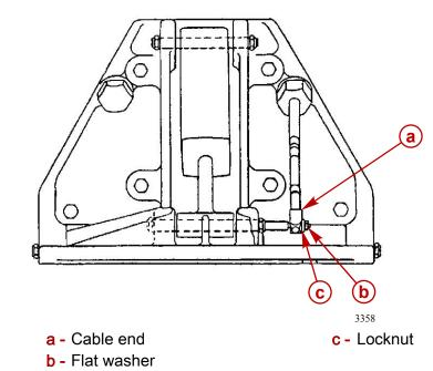
8. With the K-Plane in the maximum up position, adjust the cable so the cable end locknut is within 3.2 mm (1/8 in.)of the lower cable seal, or until the indicator reads the desired position.
