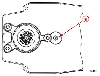
a - Control handle friction adjusting nut
