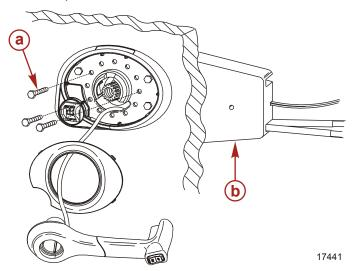
a - Control module mounting screw(3)
