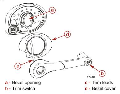
IMPORTANT: Verify trim/trailer wires are not pinched when mounting remote control module to panel of boat. Trim wires must be free to move with the remote control handle.
