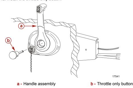
IMPORTANT: Leave the trim harness loose behind the panel. Do not use cable ties near the control module, harness must have free movement when rotating handle.
