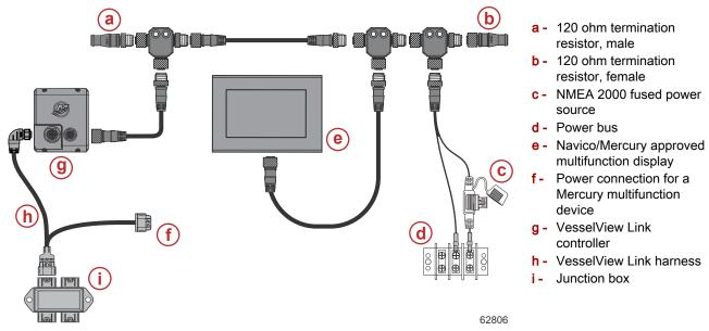
4. Connect the VesselView Link harness and the NMEA 2000 extension harness to the appropriate connectors on the rear of the VesselView Link module.
